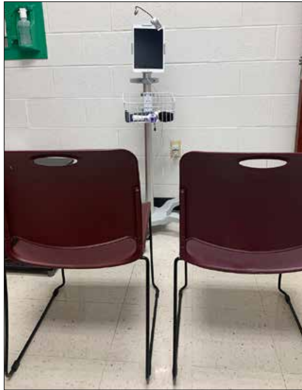
For the Intelligencer The tablet computer is mounted on a stand with casters for portability and a small basket holds typical nursing tools, stethoscope, thermometer, etc.
